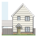
FRONT ELEVATION (WEATHERBOARDING)
